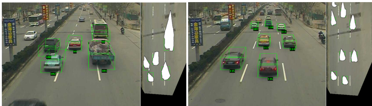
Figure 10: Fusion result of vehicle identification and tracking
