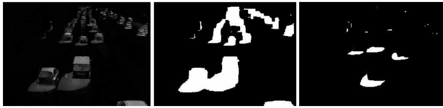
Figure 8: (a) Background subtraction result. (b) Extracted foreground. (c) Extracted shadow regions
