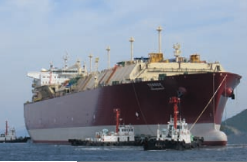
The LNG ship Tenbek is floated out of the building dock during construction in Korea for the Qatar Petroleum-ExxonMobil joint ventures in Qatar. When delivered in October 2007, this LNG ship will be the world's largest, with a capacity of 216,200 cubic meters.
