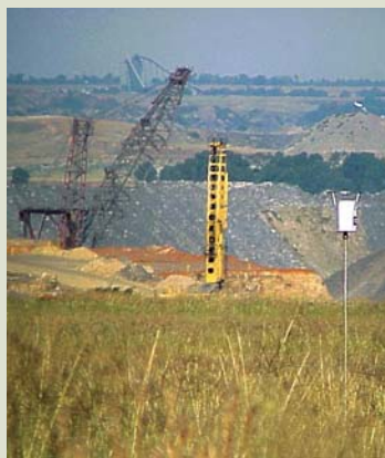
A Kleinkopje colliery dust bucket for determining dust fall out from the open cast mining operations, part of a comprehensive emissions monitoring system
