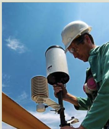
Measurement of air quality at Rustenburg Platinum Mines' Waterval Smelter
