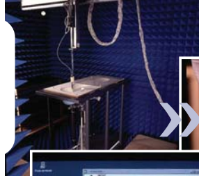
Dosimetry: a SAR test bench in an anechoic room
