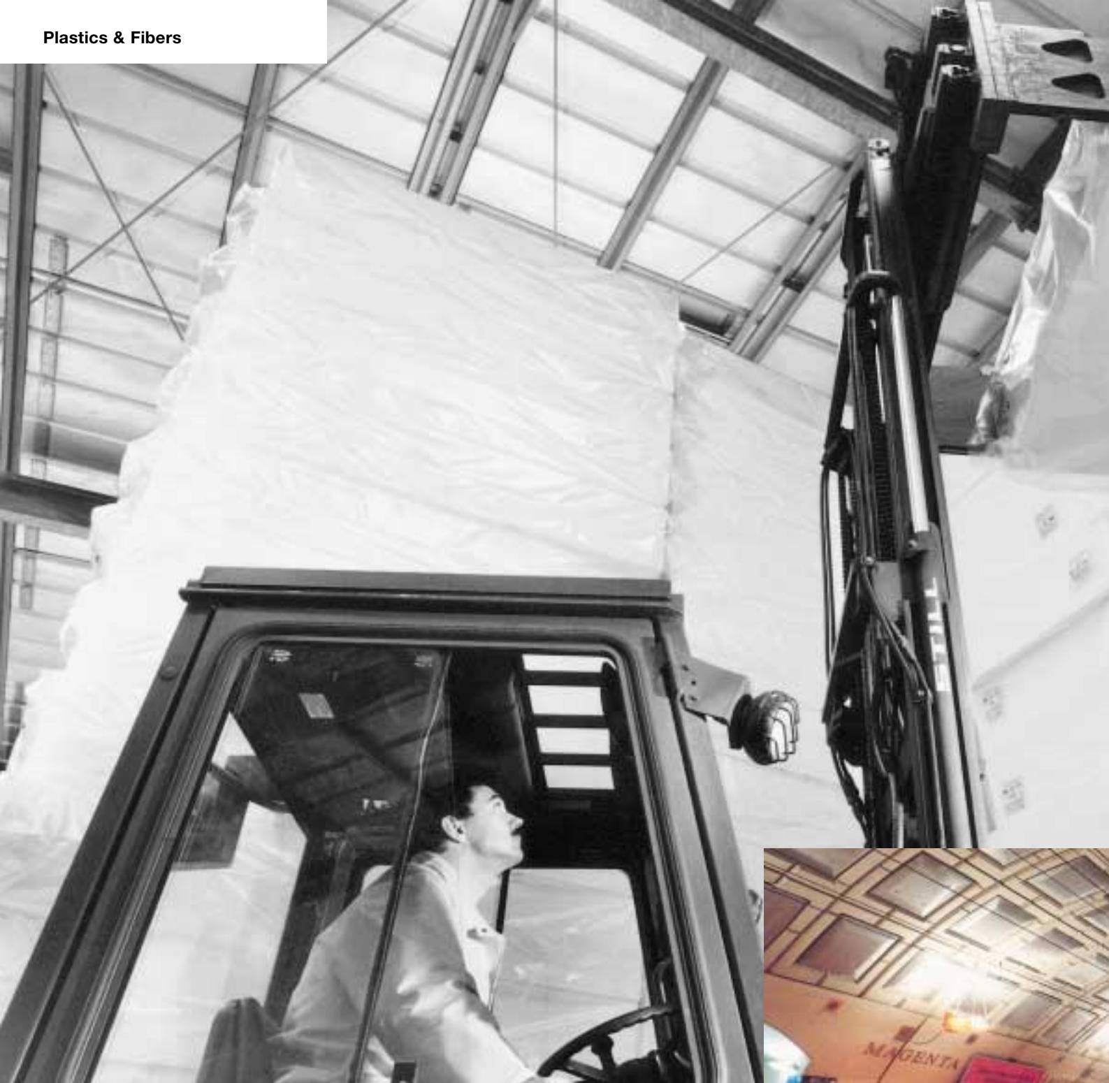
These simple-looking foam boards being stacked by Rüdiger Hahn at our site in Ludwigshafen, Germany, have a dual purpose: The BASF plastic Basotect® provides sound as well as heat insulation. It can be found in the stations of the Paris Metro.
