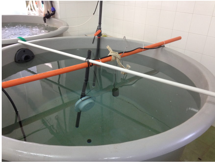
Figure 4. The equipment used for the acoustic stimuli projection in tank. The loudspeaker UW30 (left) was employed for L, ML and M frequency sweeps projection, and the cylindrical fiberglass loudspeaker (right) was used for the MH and H frequency sweeps.
