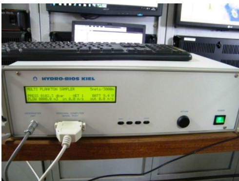
Fig. 15: MPS , “deck unit”
