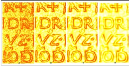
Fig. 5 – Slope models generated with different window sizes: (A) 11 grid points, (B) 25 grid points, (C) 35 grid points (D) 55 grid point.
