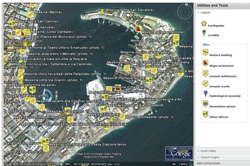
Fig. 3: EEEs induced by the December 28, 1908 Messina Straits, Italy, earthquake in the area of the Messina harbour. If information from contemporary sources is very precise, it is possible to use the EEE Catalogue also for local seismic microzonation.
