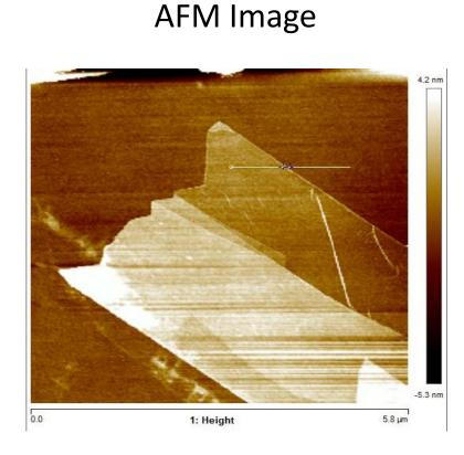
Sample thickness is measured to be ~2.5nm (shown below)
