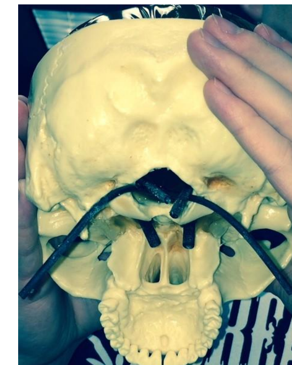
Figure 2: Inferior view of the model inside the skull. Milk is pumped upwards through the vertebral and carotid arteries into the model, and out from the top.
