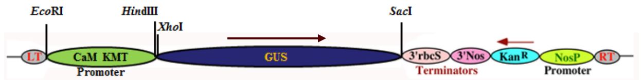
Supplemental Figure 2. Schematic diagram of the CaM KMT pro :GUS construct. All elements of the T-DNA region are shown. T-DNA left border (LT), T-DNA right border (RT), and RBCS terminator (3'rbcs). A kanamycin selectable marker gene (Kan R ) was used under the NosP promoter and NOS terminator (3'Nos).
