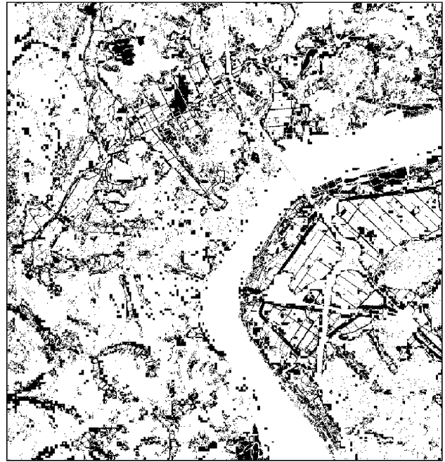
Fig. 4. Image showing the agreement of pixels in the classification of Landsat and IKONOS images. Black pixels (21% of image) were classified differently in the two images. White pixels were assigned to the same class. Image covers the same area as Fig. 2 and is 5.5 km wide.
