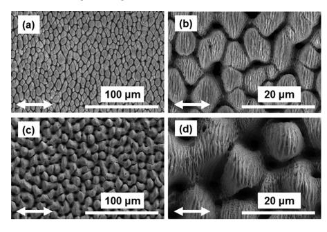
FIG. 3. SEM top surface images of BSG-mounds (a) and (b) and ASG-mounds (c) and (d). The double-ended arrow indicates laser polarization direction.
