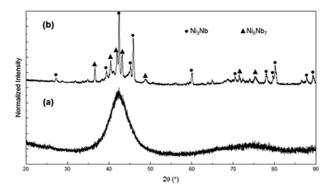
FIG. 1. XRD patterns of (a) as-solidified ribbons displaying an amorphous structure and (b) polycrystalline  $Ni_{60}Nb_{40}$  after heat treatment showing crystalline peaks corresponding to  $Ni_{3}Nb$  ( $\blacksquare$ ) and  $Ni_{6}Nb_{7}$  ( $\blacksquare$ ).
