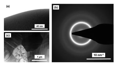
FIG. 5. (a) TEM bright field image and (b) SAED pattern of the amorphous Ni<sub>60</sub>Nb<sub>40</sub> top portion of the ASG-mound. TEM bright field image of the (c) bulk polycrystalline Ni<sub>60</sub>Nb<sub>40</sub> microstructure of the lower portion of the ASG-mound.
