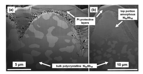
FIG. 4. SEM images of typical (a) BSG-mound cross section and (b) ASG-mound cross section.
