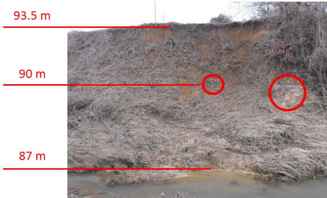
Figure 2. Dry Creek bank for seepage experiments. Photo taken January 19, 2011 after kudzu was removed. Locations of evidence of seepage are indicated by circles.
