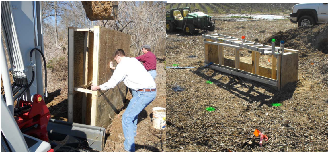
Figure 4. Trench frame installation for induced seepage experiments. The trench was located 2.8 m from the bank face.
