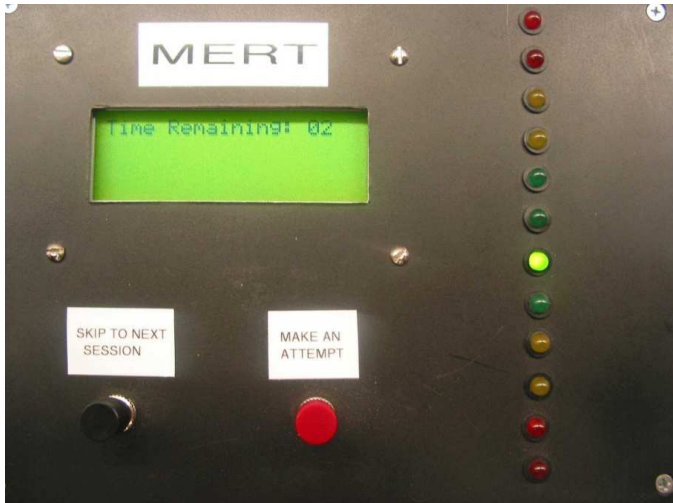
Figure 1. Existing MERT device with its monochromatic LCD, two button interface, and large form factor.
