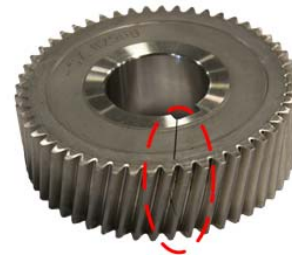
Fig. 8. The test gear with a crack.
