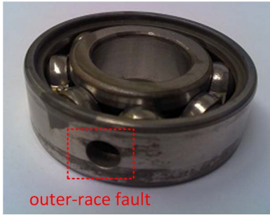
Fig. 12. Test bearing with an outer-race fault.
