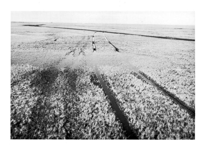
Photograph 1. Tracks of Weasel (M 29C), left, and of an LVT, right, crossing tundra near Point Barrow. The Weasel rides on the surface without breaking the vegetation mat. The LVT breaks through and rides on the permafrost table. Heavily traveled tractor road in the background. (U. S. Geological Survey, 1955.)
