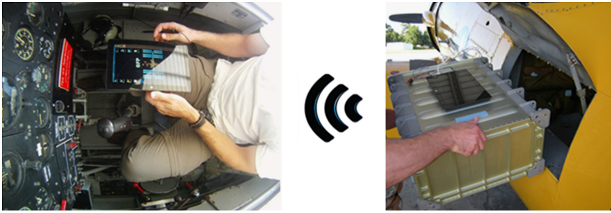
Fig. 5. Wireless tablet control of the Flex Imager. The MDL mounted tablet was hardwired, to the internal USB hub and configured to distribute a wireless network (right). The tablet remained affixed to the MDL during flight, such as when the MDL was installed in the T-6 rear baggage compartment. The operator controlled tablet is connected to this configured wireless network and utilized to actively control the hardwired tablet and payload (left).
