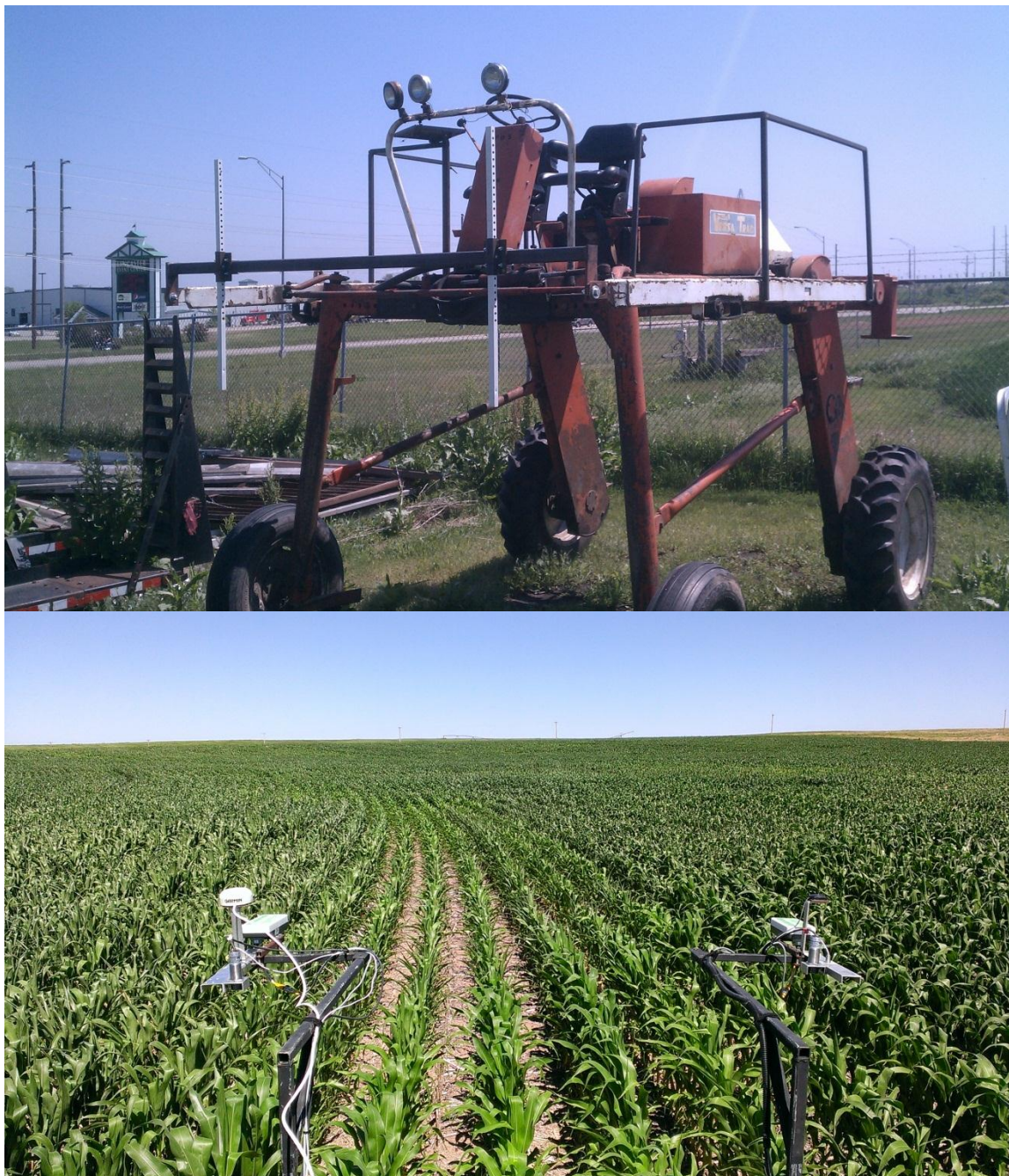
Figure A-8 Image of high clearance machine used to collect data in 2012 and 2013 (above) and high clearance machine with sensors attached collecting data at the Brule Water Lab site in 2013 (below).
