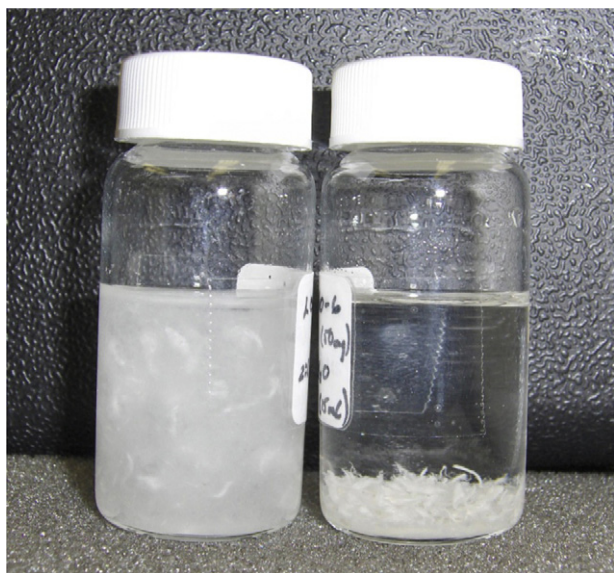
Fig. 11. L040-6 (left) and PL0406-T (right) mixed in 50% by mass ethanol–water solutions.
