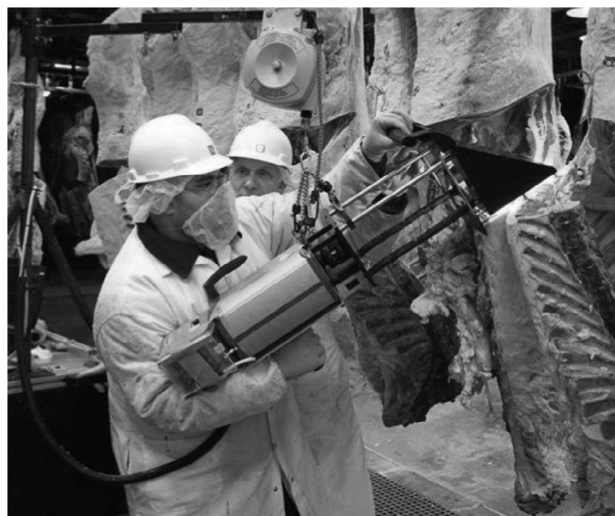
Figure 2. Acquiring image of beef ribeye using the prototype on-line acousto-optic tunable filter (AOTF)-based hyperspectral imaging system (HSI).
