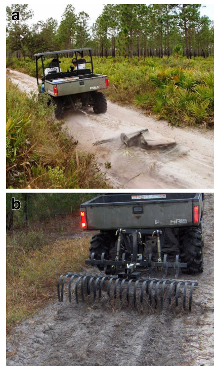
Fig. 2 Preparation of tracking plots using a drag device ( left photo ) and mechanical rake ( right photo ) to smooth the track plot surface
