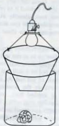
Figure 13 - A simple "white" light trap for collecting night-flying insects.
