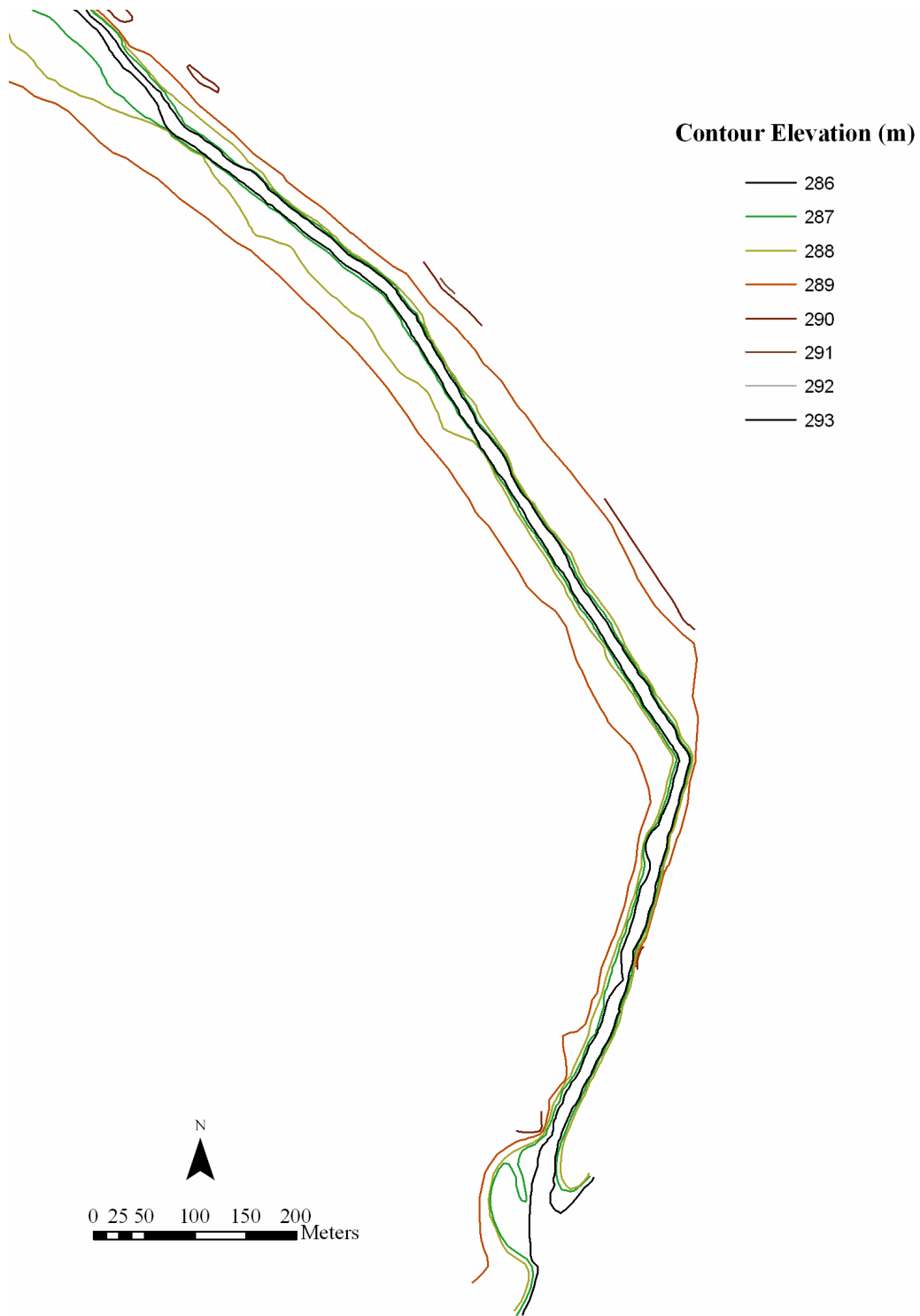
Figure II.4.4. Topographic survey of the lower quarter of Tobacco Island.
