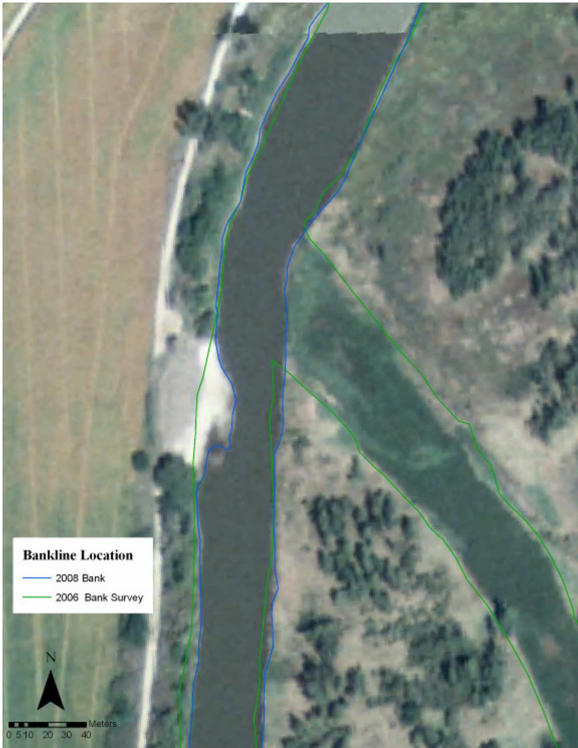
Figure II.3.5. Close up of sloughed bank with bankline locations from 2006 topographic survey and 2008 aerial photography.
