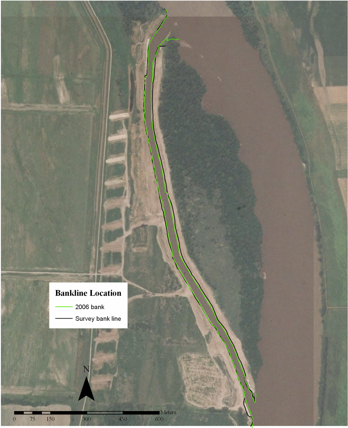
Figure II.8.2. Aerial photograph of Kansas (lower) with bankline locations from 2006 aerial photography and the topographic survey.
