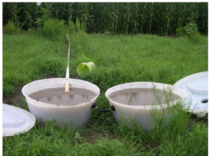
Figure 1. Runoff tanks for collecting water samples after each runoff event
