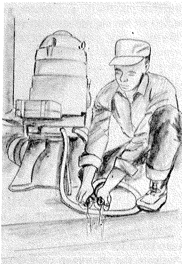
DRAIN WATER FROM GEAR HEAD
