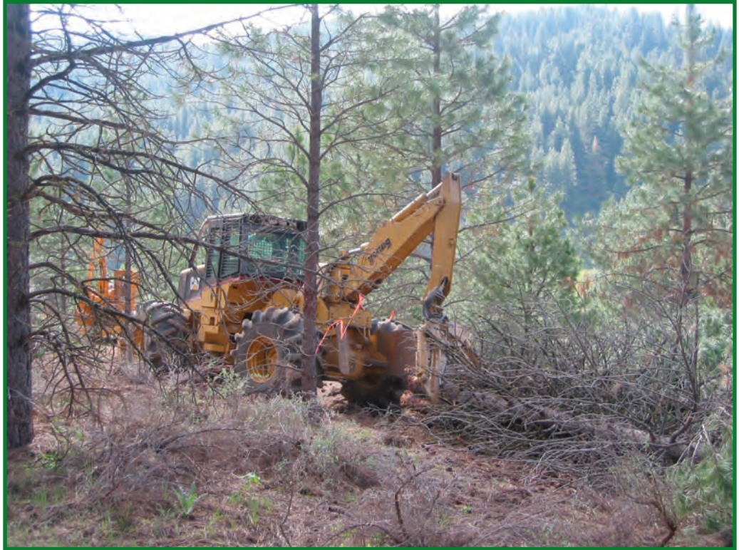
Figure 8.9. Skidder extracting whole trees to a landing where trees are processed into sawlogs or biomass for energy production.
