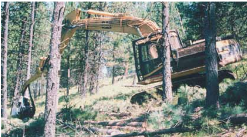
Figures 4a–b. Mechanical thinning operations. At left, a harvester performs a mechanical thinning operation in the Northern Rockies. (Andrew Youngblood, USDA Forest Service, cfc.umt.edu) At right, a forwarder works at the Blue Mountain FFS site in northeast Oregon. (Elizabeth Dodson Coulter)
