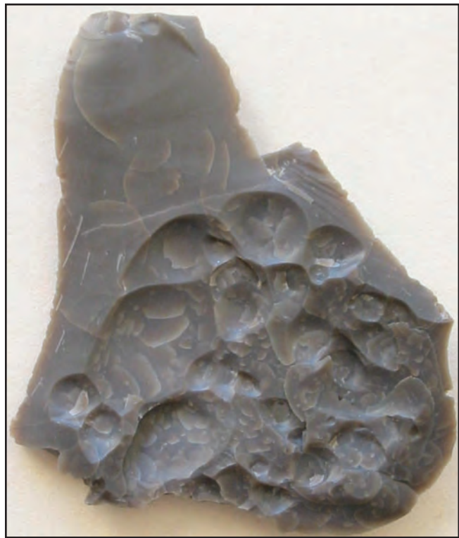
Figure 4-1 —Potlidding, crazing and cracking on chert thermally damaged during a heat-treatment replication experiment (sample courtesy of Rob Jackson).
