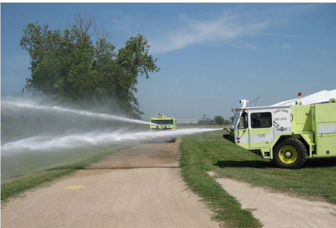
(Above) NFS mechanics test the water flow capacity of recently acquired excess federal property before transferring the equipment to a volunteer fire department.
