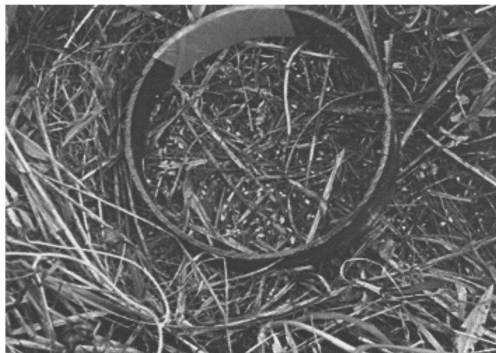
Figure 3. A sampling frame used in moist-soil habitat to prevent collection of seeds outside the sampling area during vacuum sampling.
