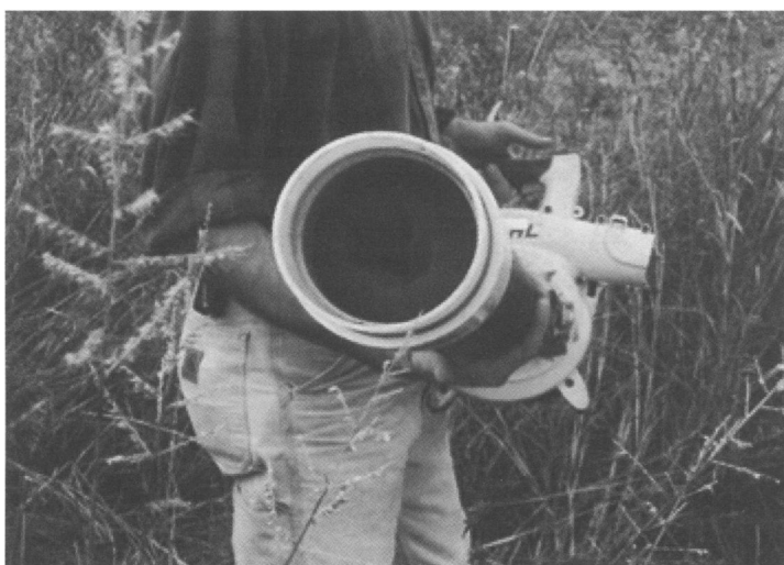
Figure 2. PVC couplers attached to the Stihl BG-85 hand-held blower vacuum, showing inserted nylon stocking that collected seeds and debris during vacuum sampling.
