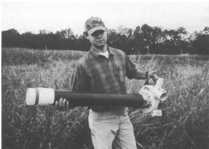
Figure 1. A blower-vacuum sampler (Stihl BG-85) used to estimate abundance of moist-soil plant seed mass.
