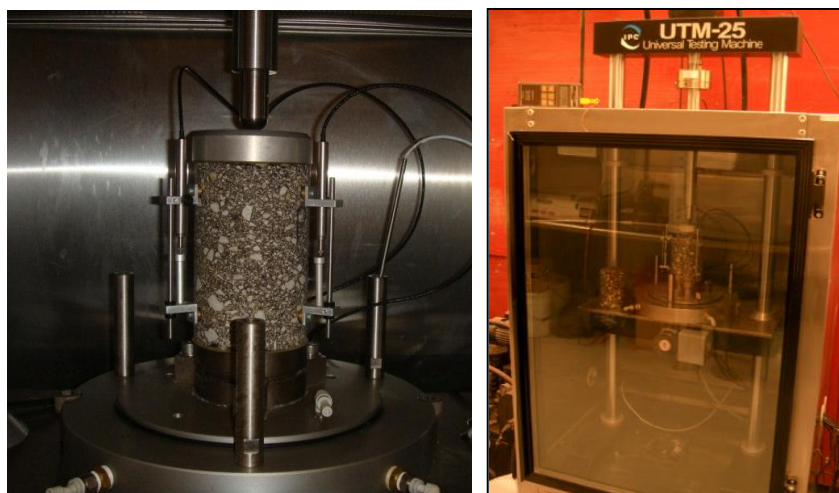
Figure 3.7 A Specimen with LVDTs mounted in UTM-25kN Testing Station
