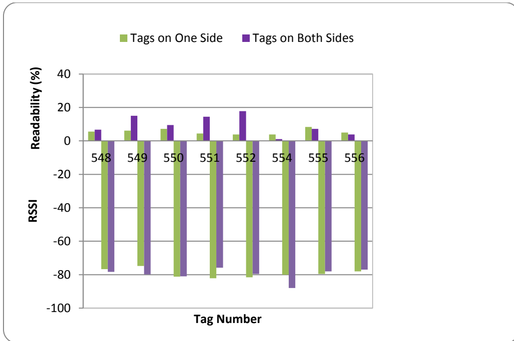
Figure 5.9 Signal Strength for Tags at 4 ft on Delineators and Signposts for Dynamic Testing
