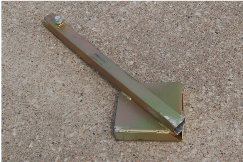
Figure 85. System Damage, Test No. WZ09-3B
