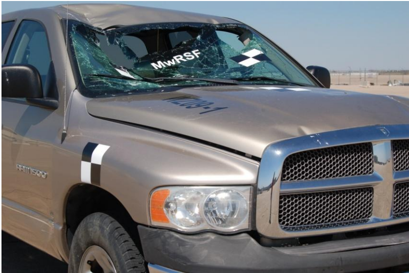
Figure 58. Vehicle Damage, Test No. WZ09-1
