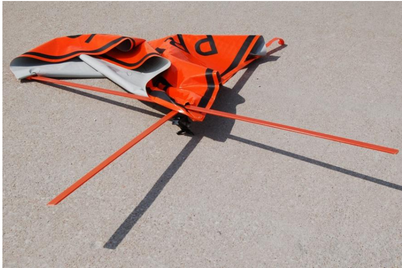
Figure 96. System Damage, Test No. WZ09-4A
