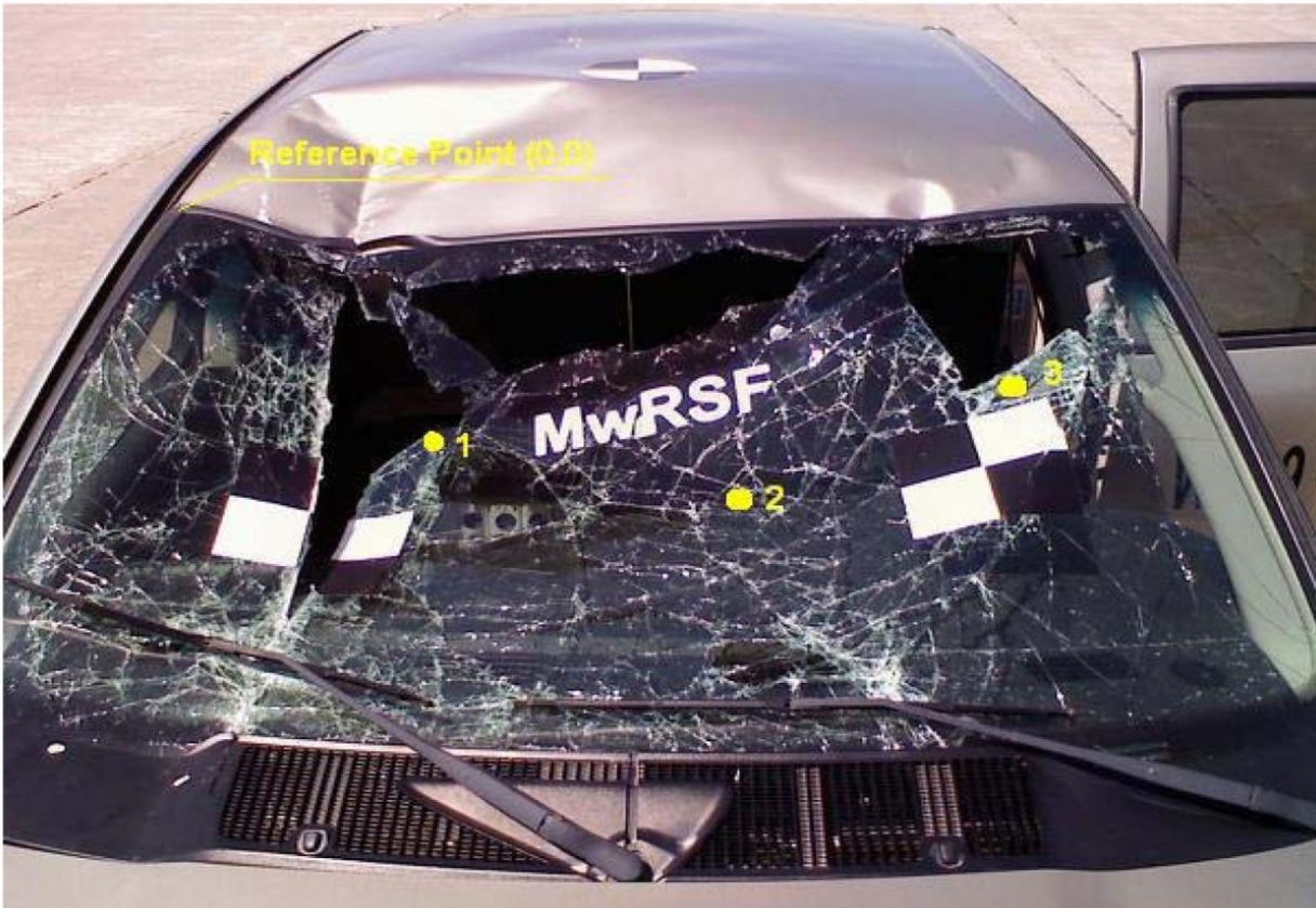
Figure E-2. Windshield Deformation Data, Test No. WZ09-1
