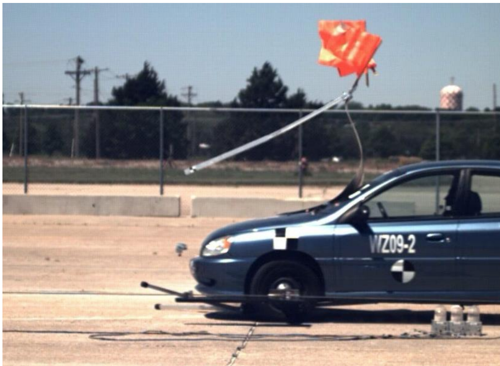
Figure 103. System No. 3A, Frangible Mast
