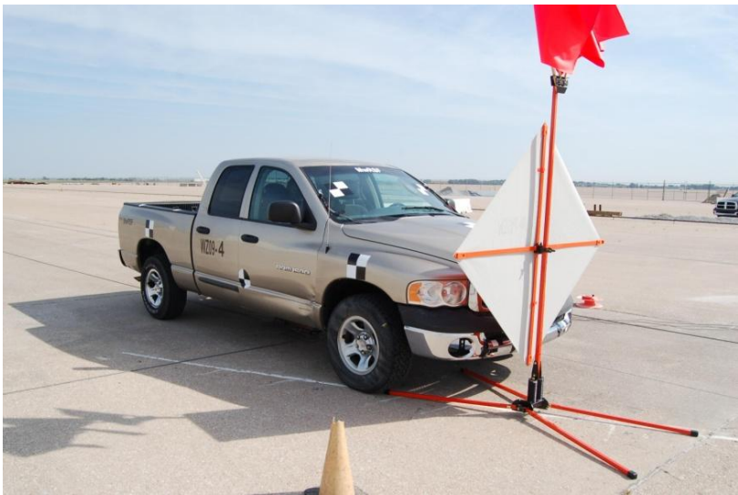
Figure 93. Impact Location, Test No. WZ09-4A
