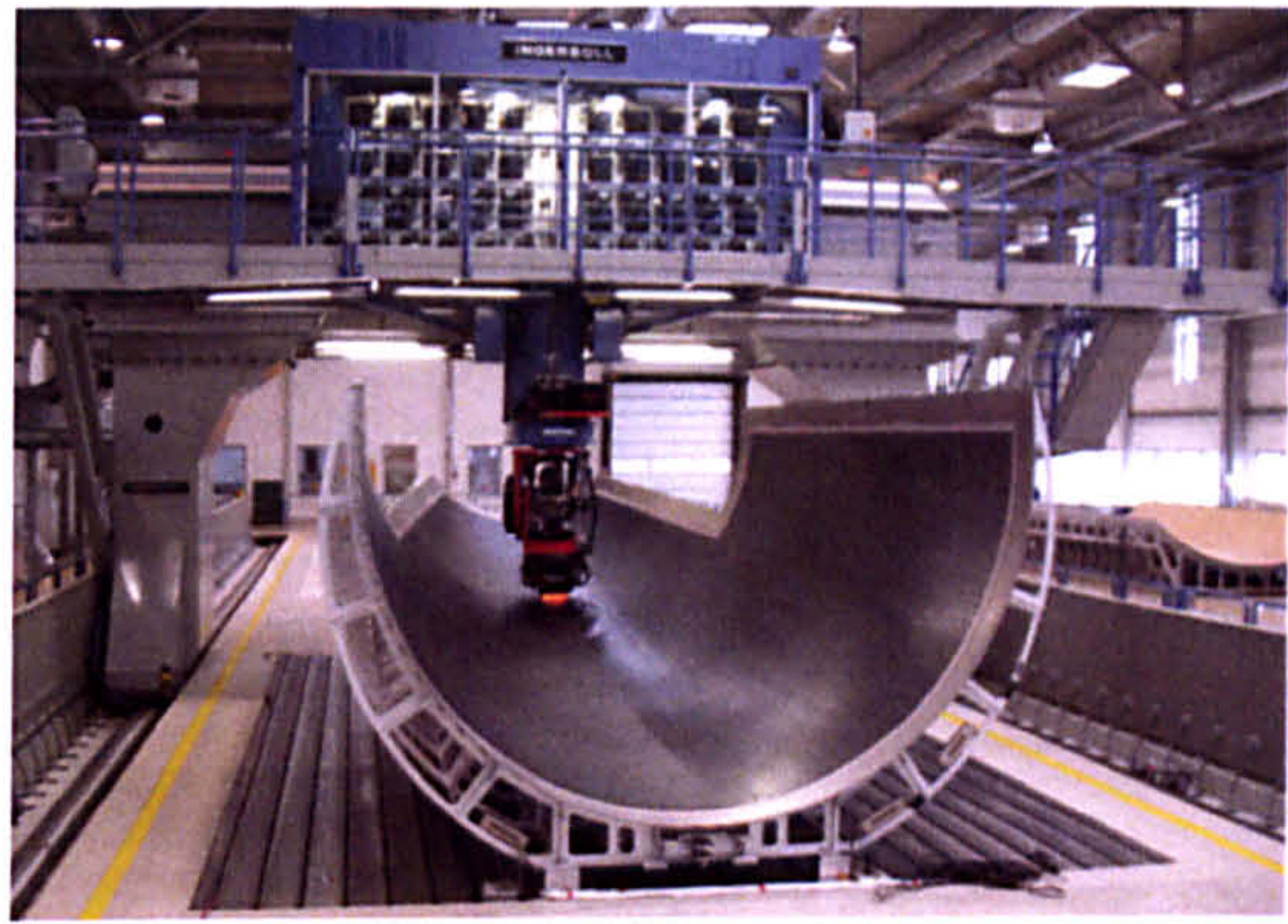
Figure 11: Ingersoll gantry-type AFP laying into a female mould, from [5].
