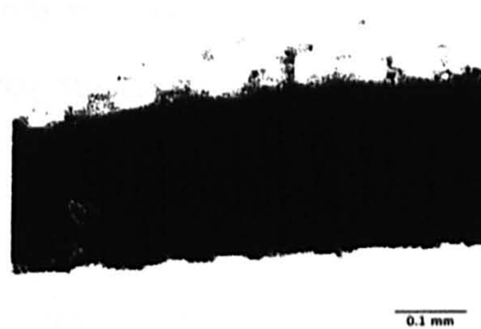
Figure 58: Sample area coloured black after digital image analysis. Note that voids are counted towards the total sample area.
