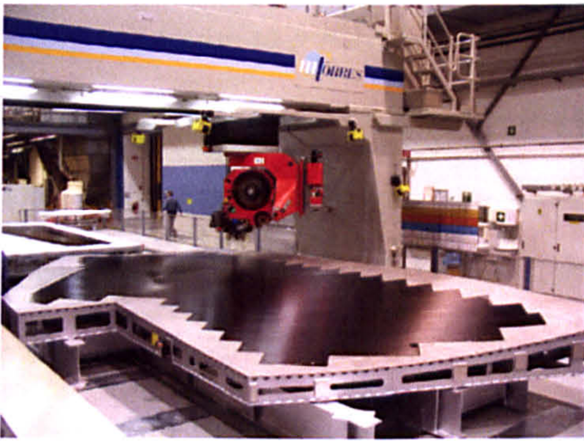
Figure 3: Example of a gantry type ATL laying onto a female tool.
