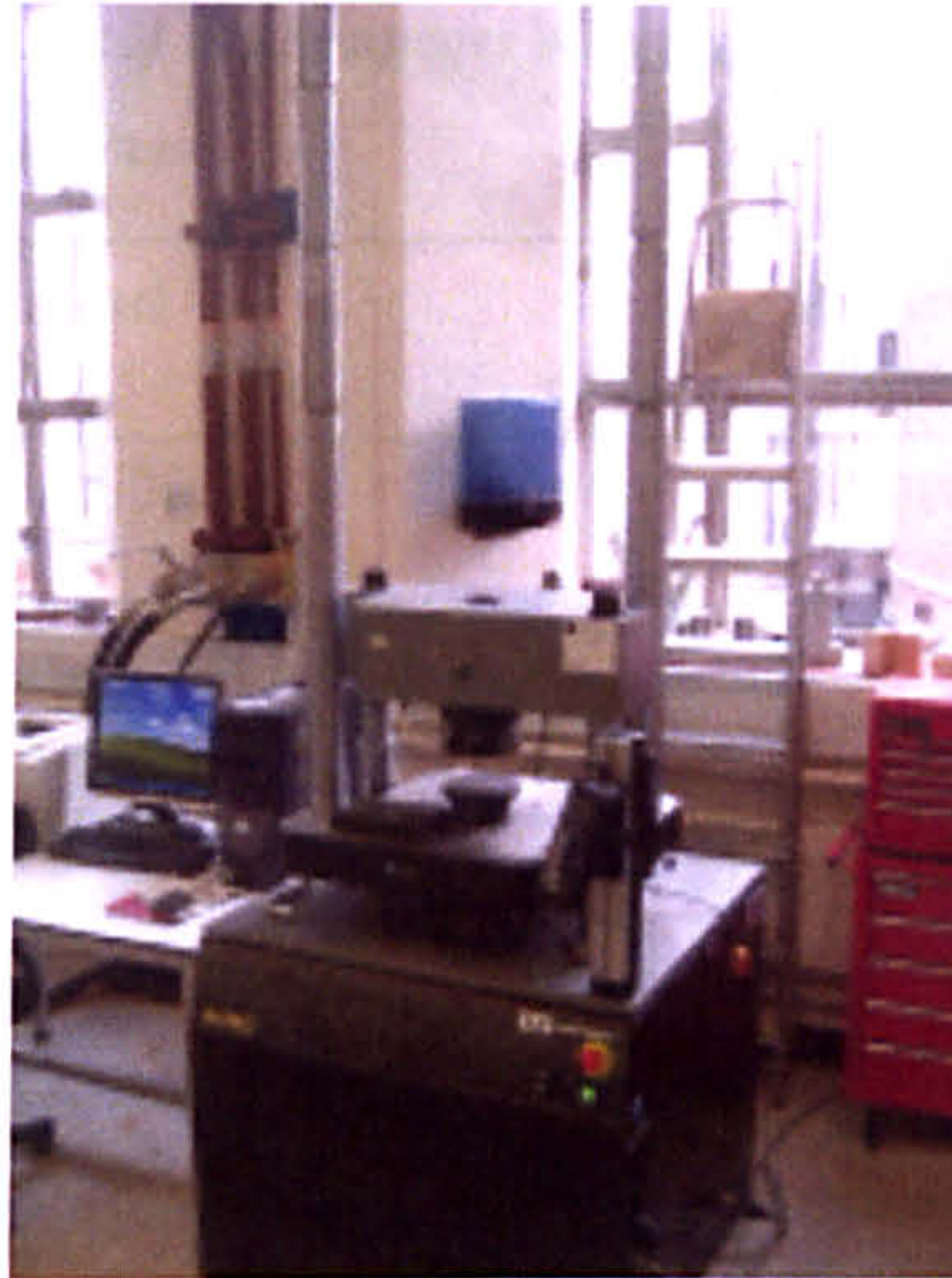
Figure 44: Picture of the Instron Satec 600DX showing the compression and tension section
