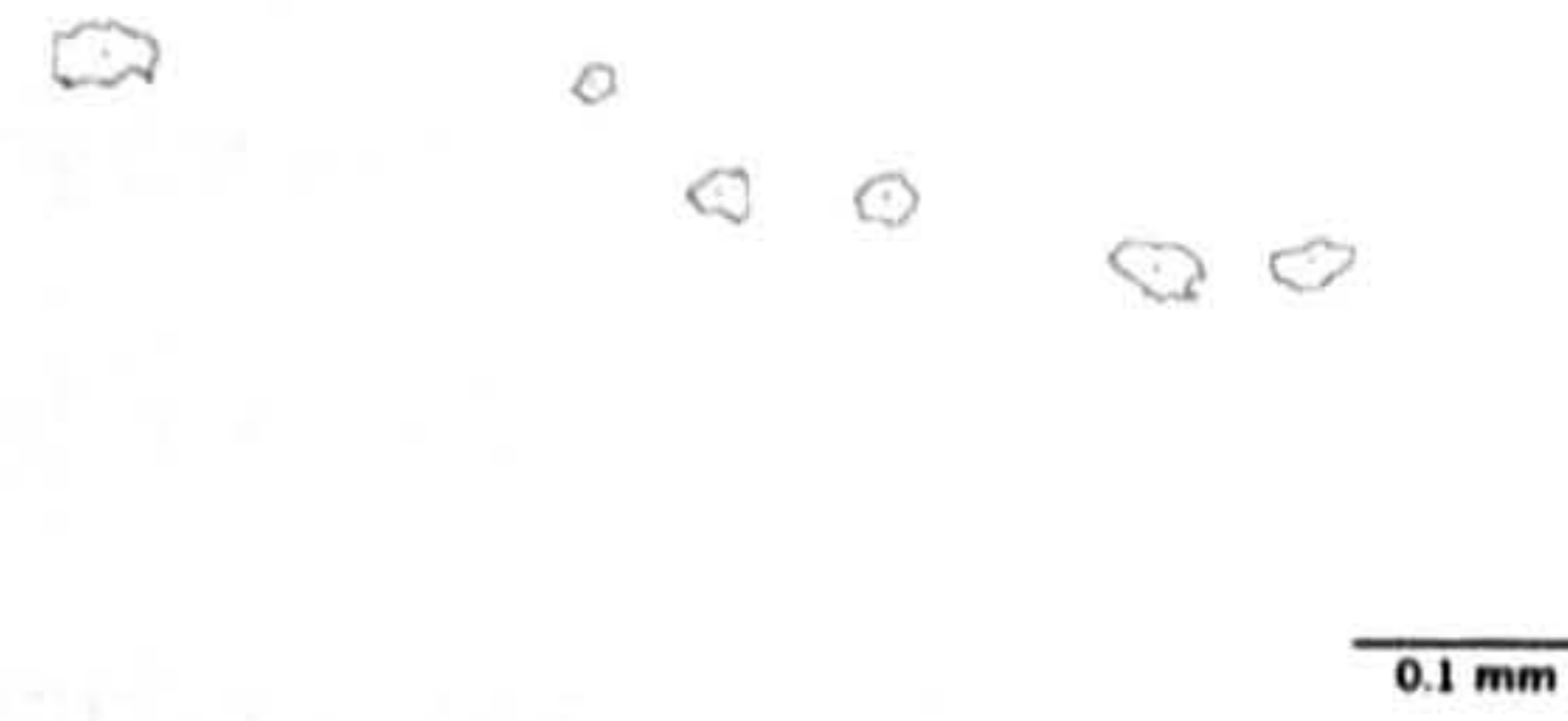
Figure 60: Void area after counting. The outlined area is counted towards the void area.
