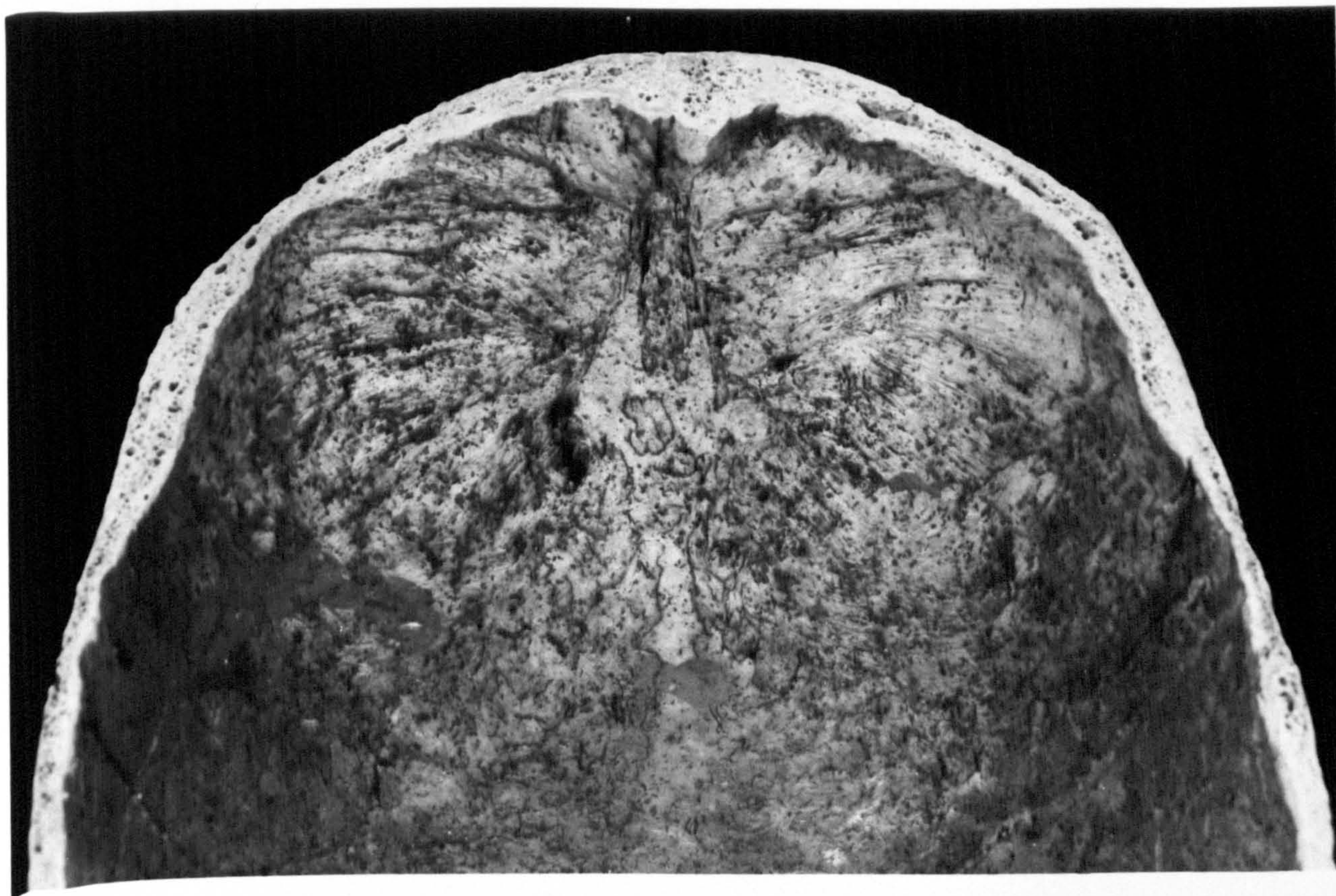
Figure 5.6 X-ray appearance and visual appearance of grade 3 HFI
