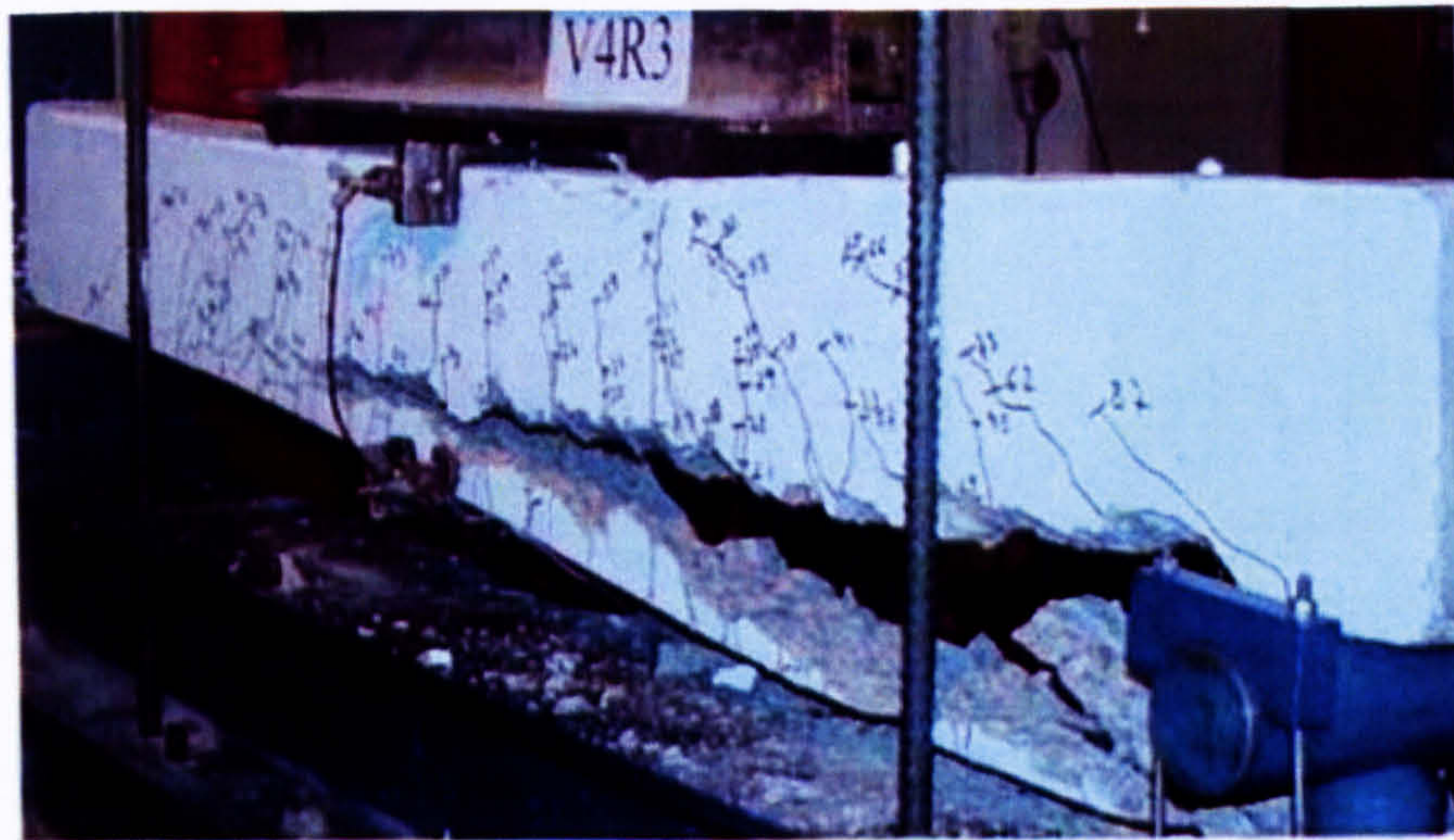
(c) Separation mode I of concrete cover
