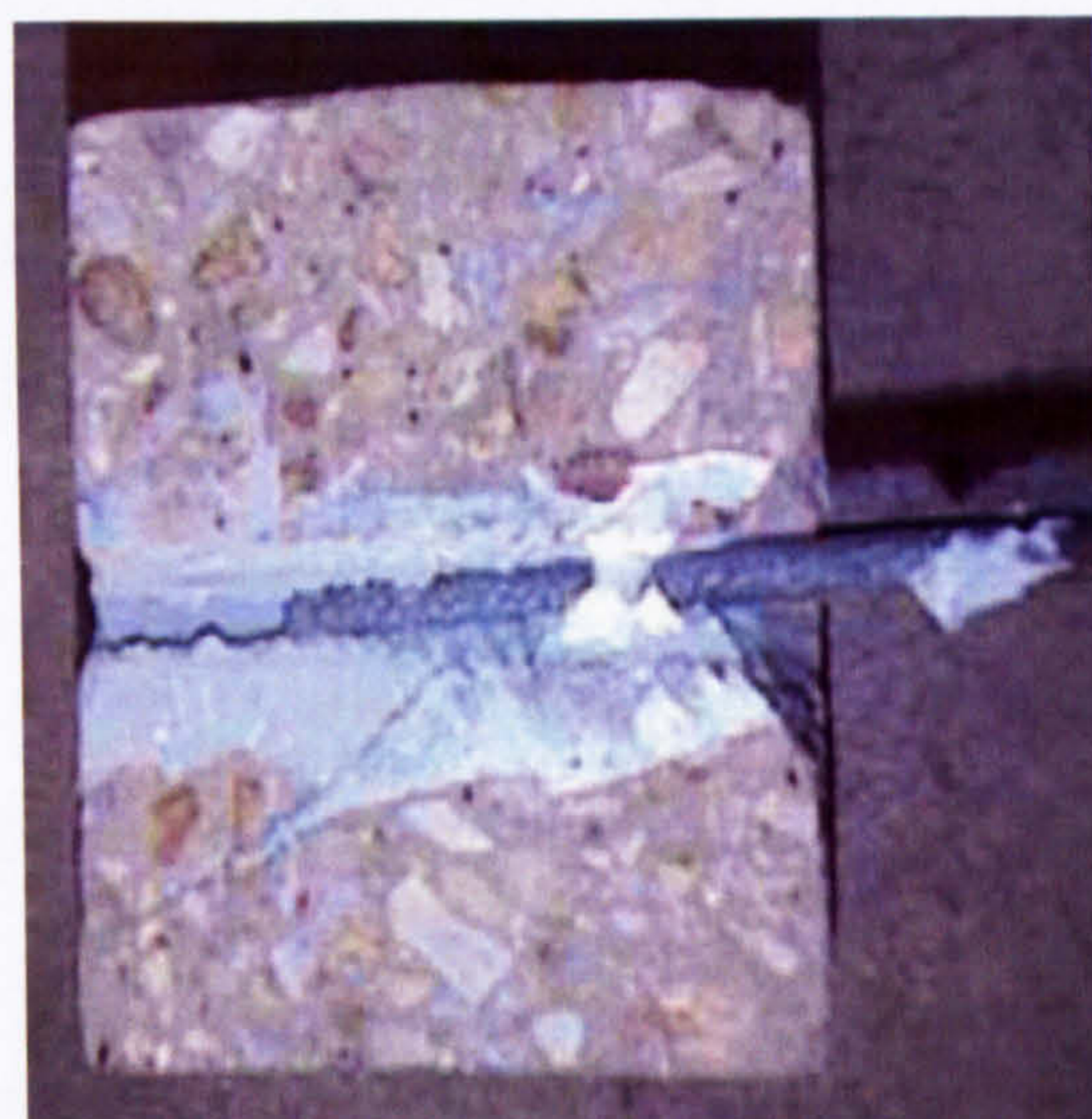
(b) Failure in bar-epoxy interface
