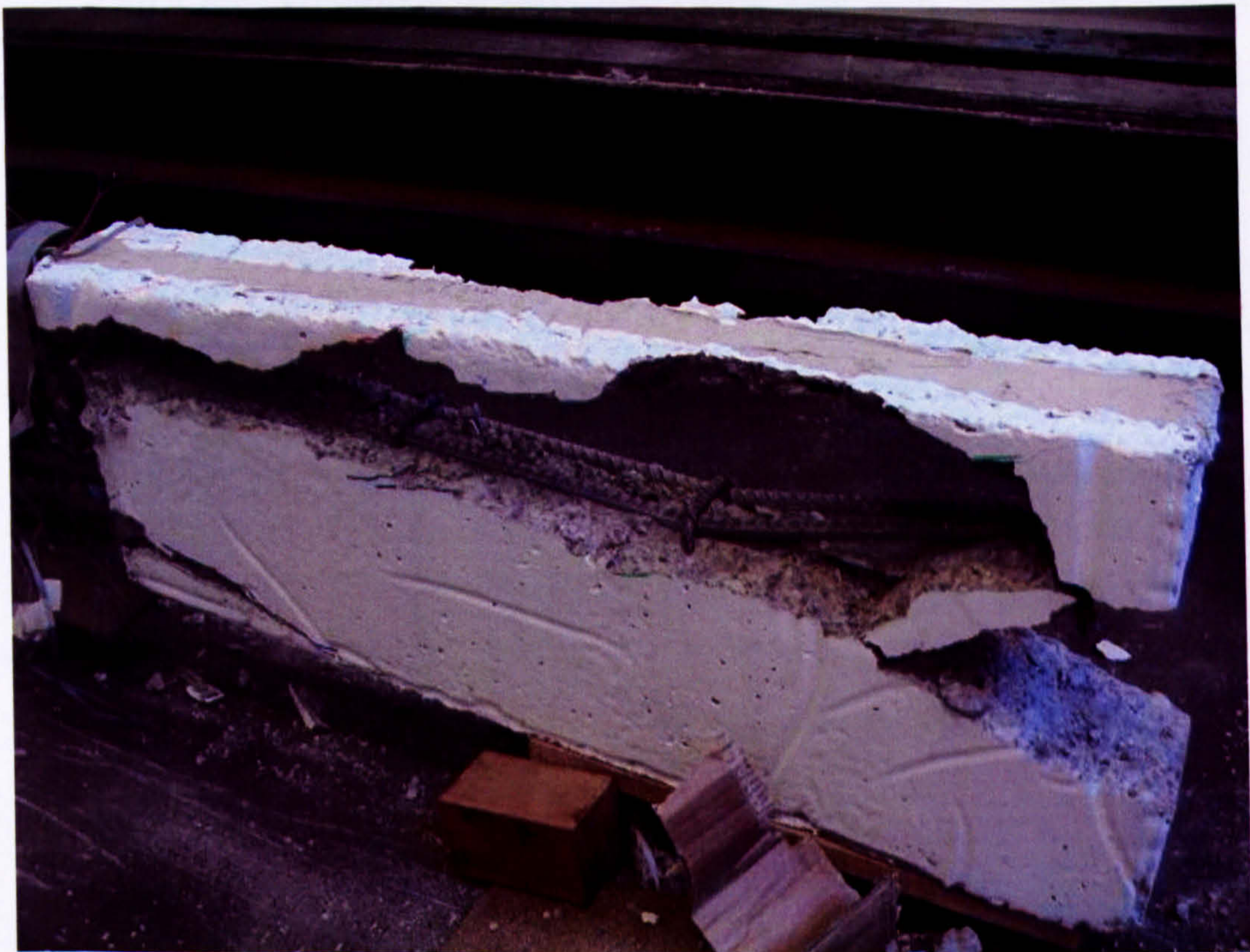
(b) B4 (fracture of end concrete block)
