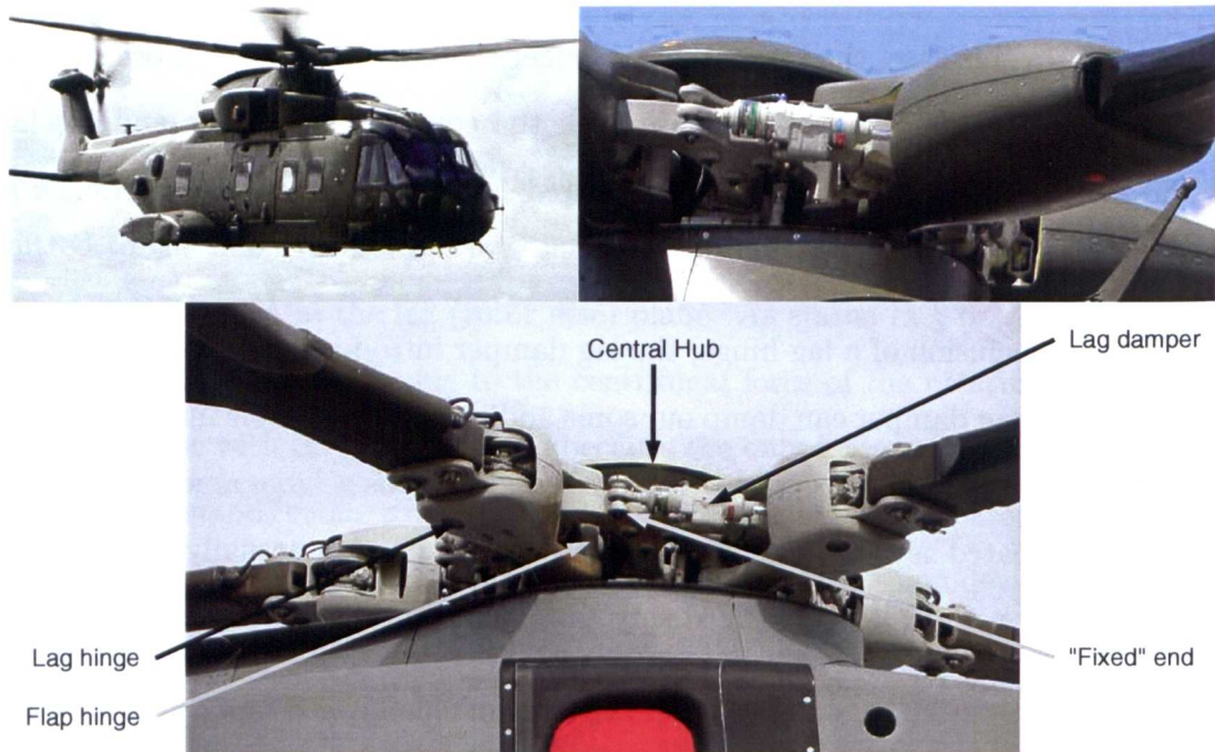
Figure 6.2: Close-up of the EH101 hub rotor system.
