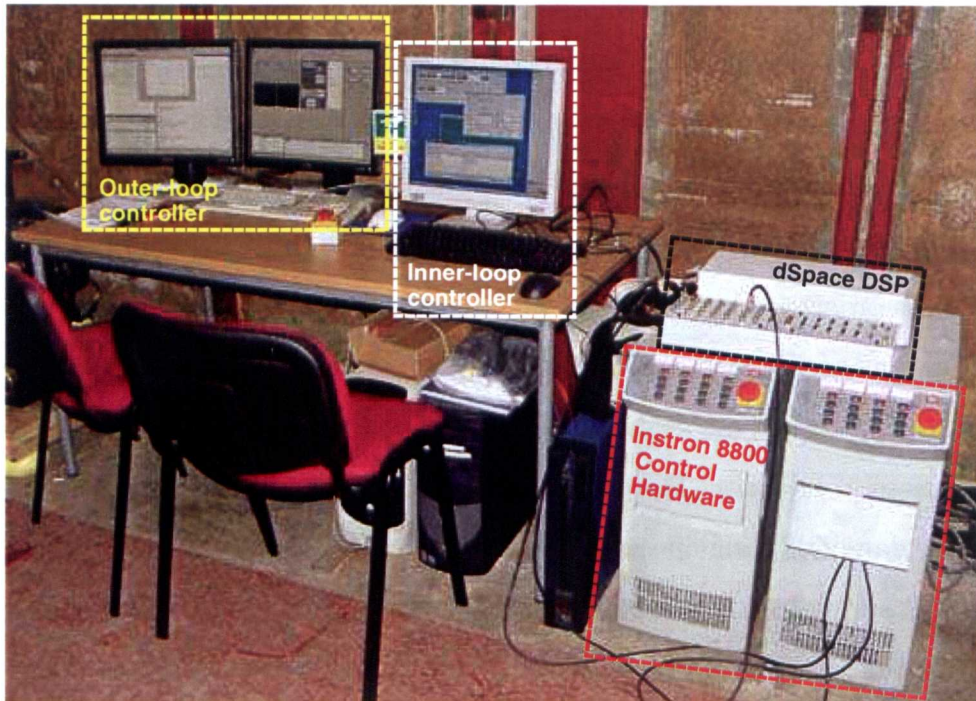
Figure 6.6: Experimental test rig controller station; 4 components: 8 channel Instron 8800 hardware control system, dSpace 1103 DSP processor and expansion board, Inner-loop control computer and Outer-loop/substructuring algorithm computer.
