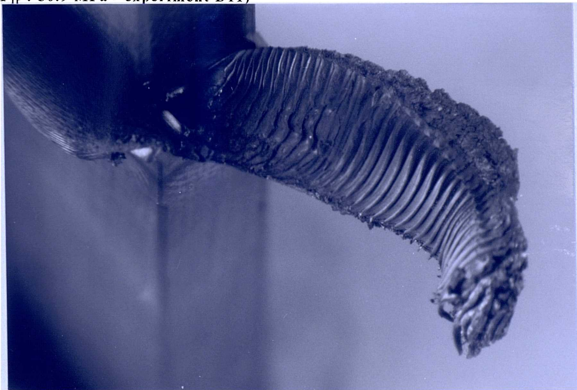
Figure 117 . Detail Of Ridged Flash Of Linear Friction Weld (Ti 6Al 4V, \alpha : 3 mm, f : 19 Hz, P_{fr} : 40.9 MPa - experiment A13)
