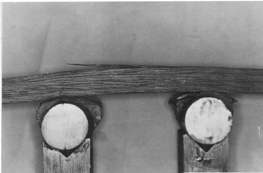
Figure (10.1) Photo of tensile cracks of a sliced Khaya specimen at 3 million cycles.
