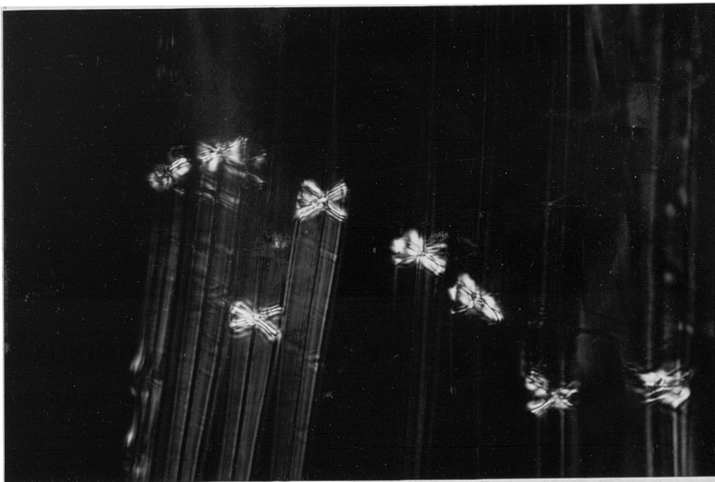
Figure (10.10) Higher magnification view of the compression failures from the central portion of figure (10.9).
