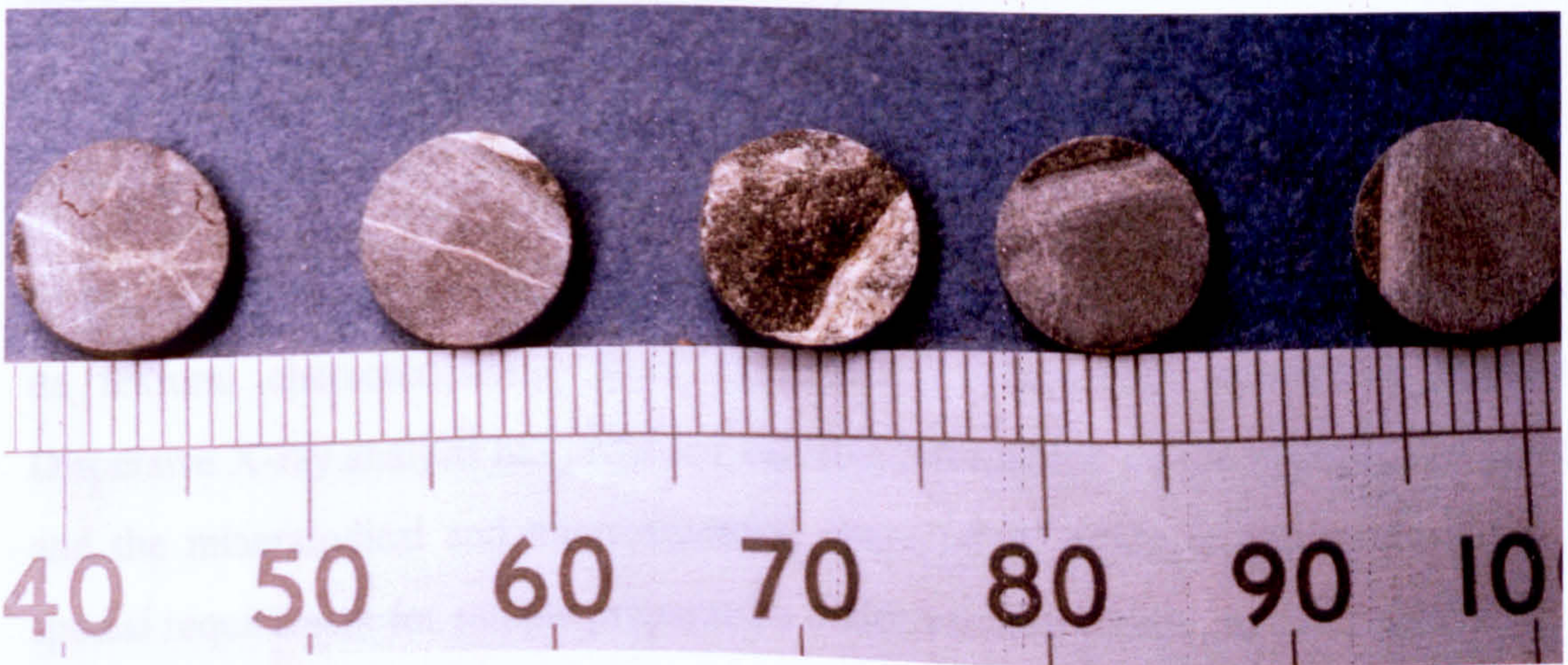
Figure 3.7 Thin rock tablets that were used for spectroscopic observations, allowing faster solution penetration.
