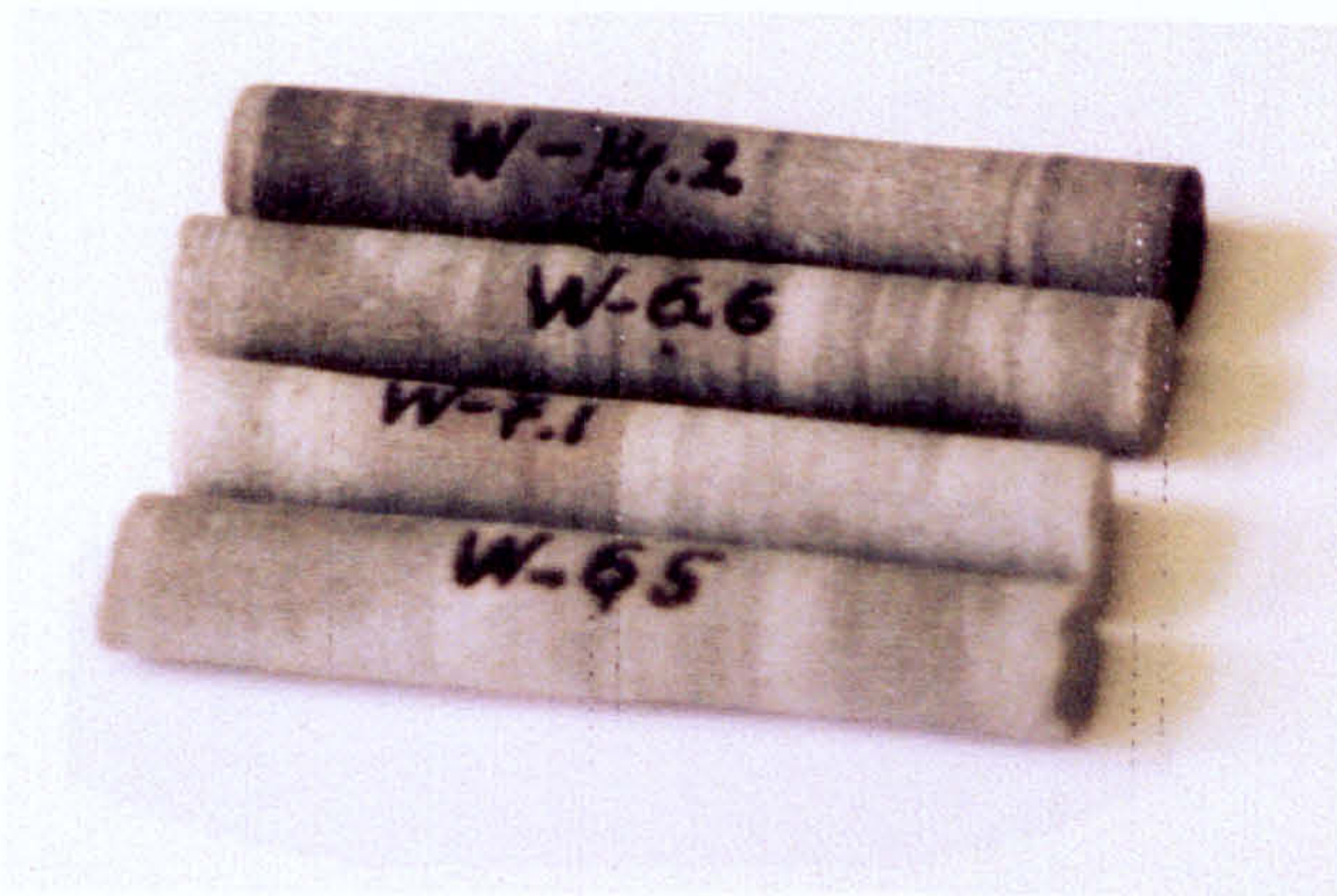
c) rock cylinders (5-6 cm length, 9mm diameter)
