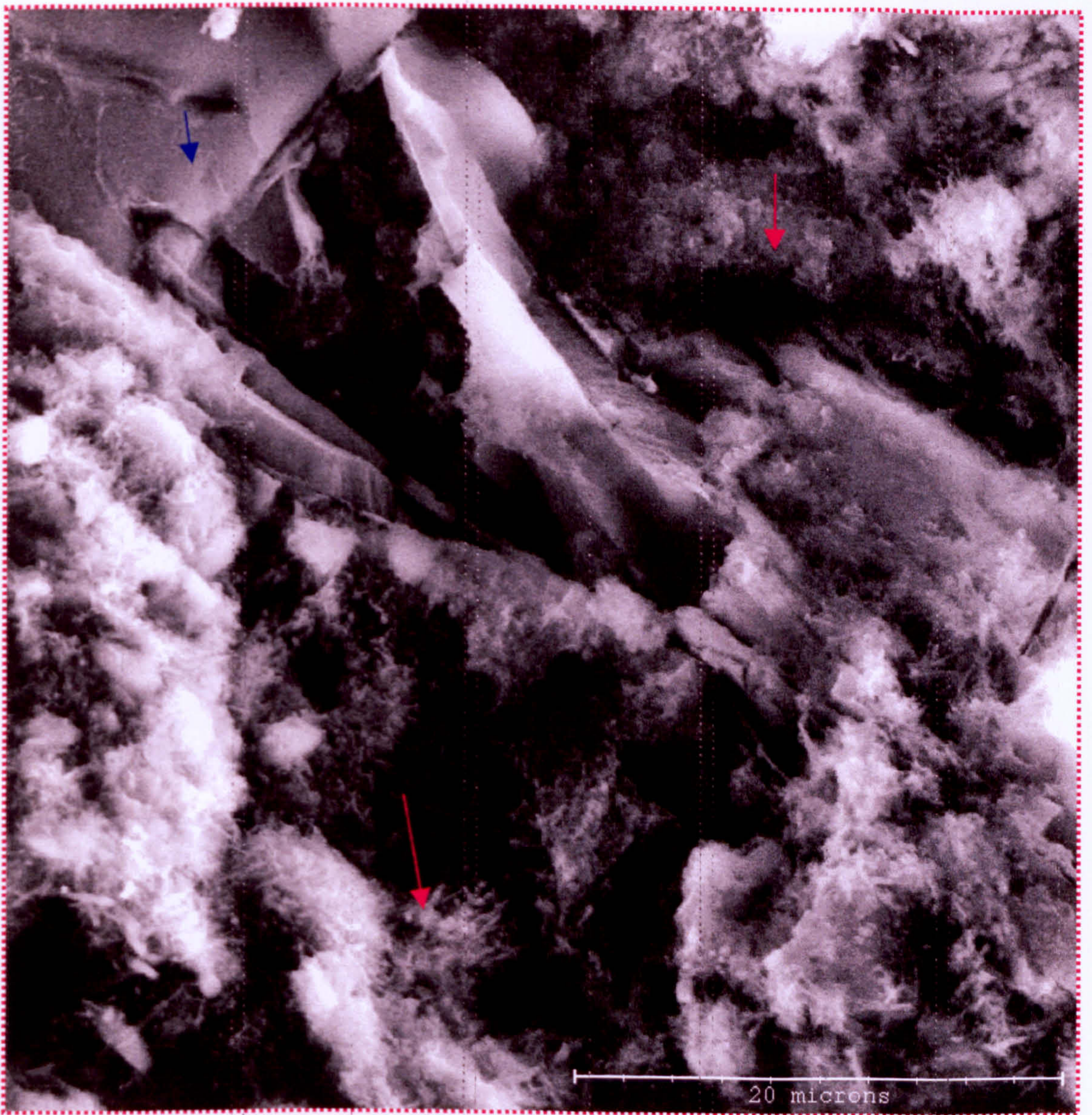
Figure 7.12 ACR affected concrete sample from Canada with Kingston dolomite as aggregate, ESEM enabled detection of a very fine deposits.
