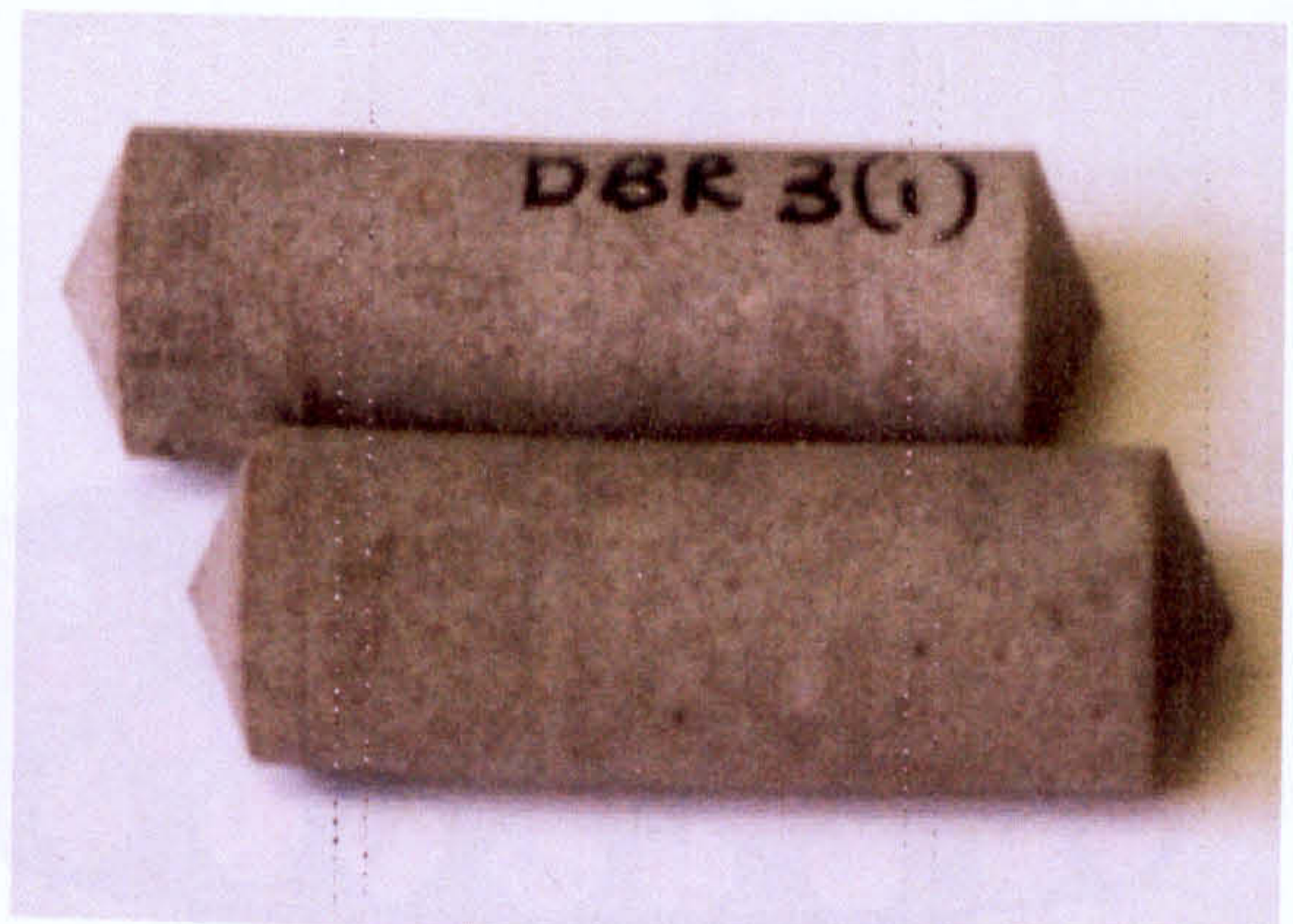
d) cone-ends (angle 120^{\circ} )(ASTM C586) 35mm length
