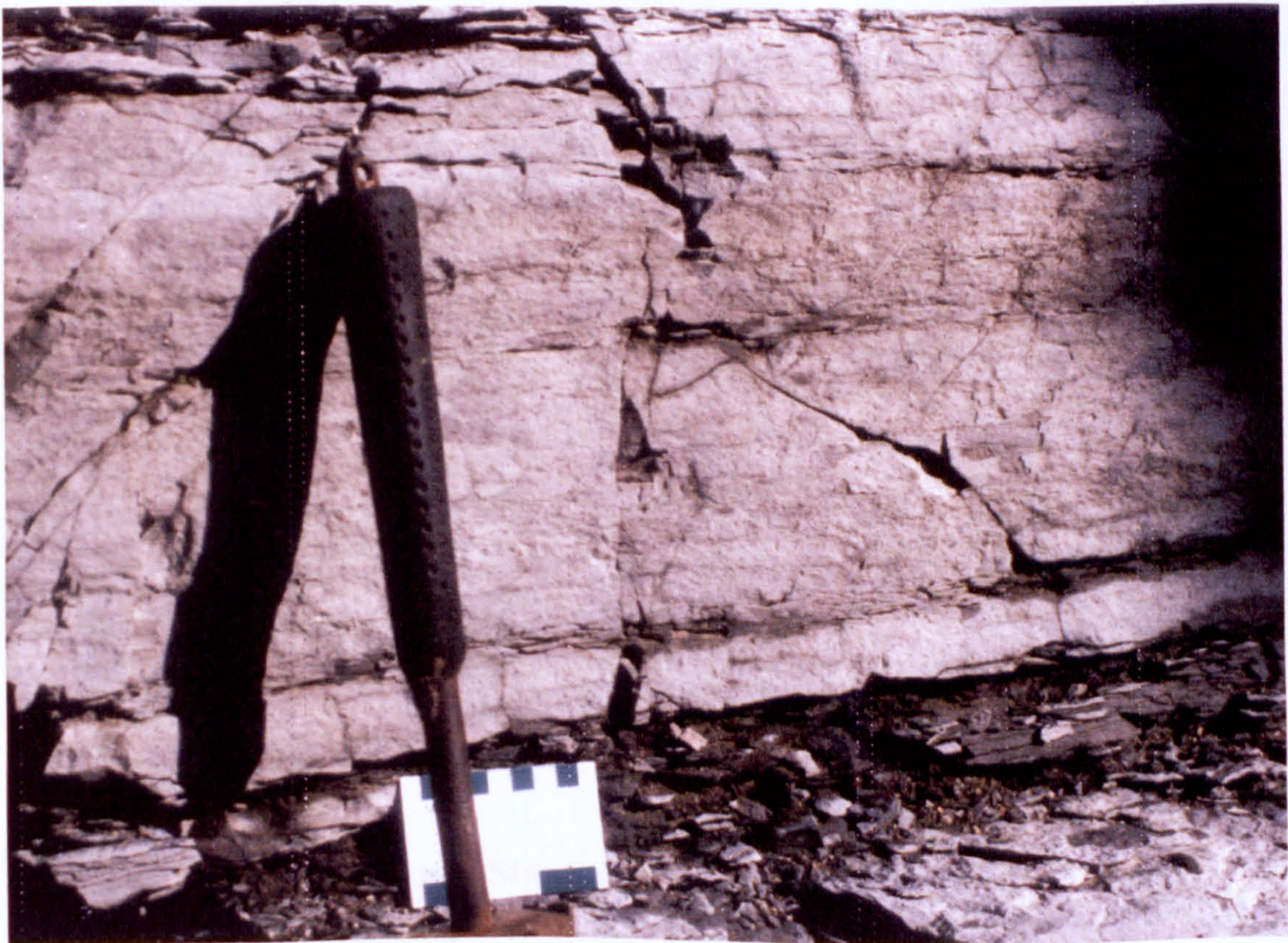
Figure 3.1 Pittsburg Quarry, Kingston Canada. Top image displays a layered formation of argillaceous dolomitic limestone showing expansive (grey) and non-expansive (pale brown and green layers). Lower image shows a close-up of the expansive layer.
