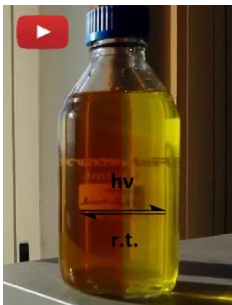
Video 2. Sunlight driven activation of 1 L of meta-stable state photoacid solution, as shown by the photochromic transition from red/orange (left, high pH) to yellow/green color (right, low pH). https://youtu.be/m_WfybTrEB8 and http://dx.doi.org/doi.number.goes.here
