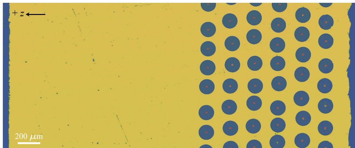
Figure 4. False-color SEM micrograph of MMC-Ti laminate cross-section. Note that the image is perpendicularly oriented to the sketches in Figure 3.
