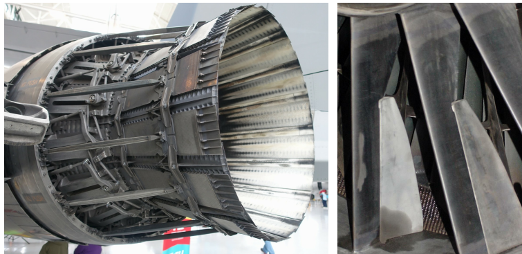
Figure 1. Two examples of the mechanism approach towards variable geometry gas turbine components. Pratt & Whitney F100 variable exhaust nozzle, and Pratt & Whitney J58 variable inlet guide vane (silver blade), which pivots aft of the black-colored static guide vane.
