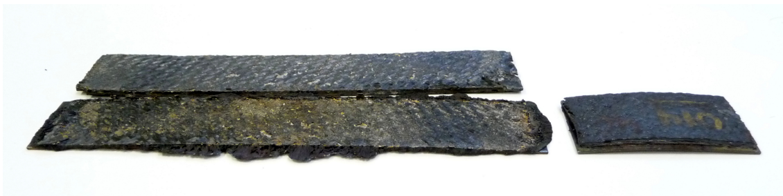
Figure 8. Photograph of debonded braze interface (left) and successfully joined laminate (right). Note the curvature that has developed in the joined laminate.
