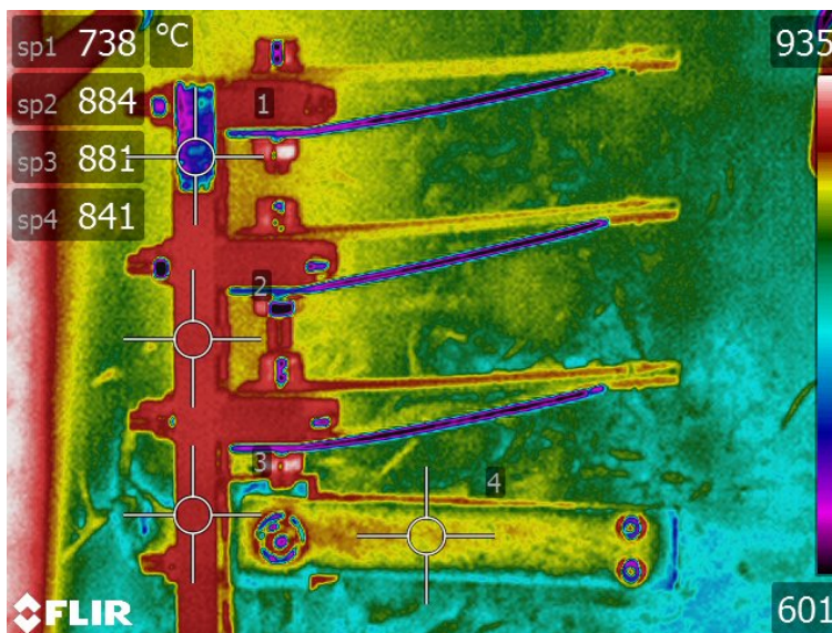
Figure 12. Thermal imagery data showing several CMC-metallic flap section thermal morphing test articles. The regions of markedly lower apparent temperature ( T < 800^{\circ}\text{C} ) are areas where bare metal is exposed, which due to its relatively low emissivity, appears cooler to the thermal camera.
