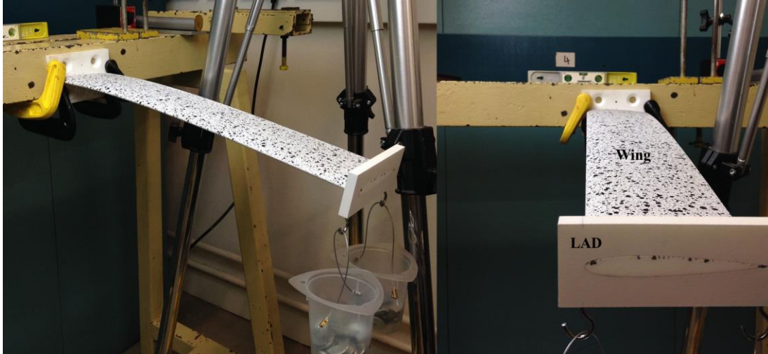
Figure 6. Load Application Device (LAD).
