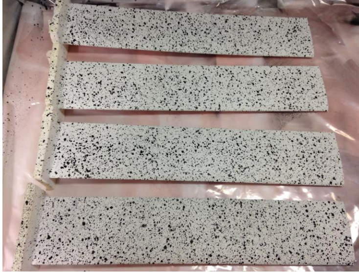
Figure 5. Illustration of the Black Speckle Pattern Applied on the Wings.
