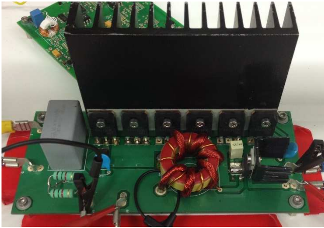
Figure 3. Experimental circuit. Top: schematic diagram. Bottom: Experimental hardware. No forced cooling is required.
