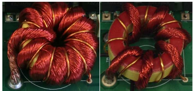
Figure 6. Photographs of the modified (left) and original (right) snubber inductors.
