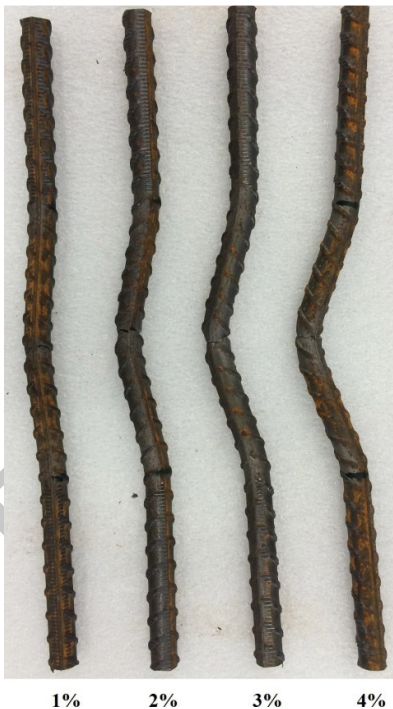
Fig. 6. Control bars with L/D = 10 after low-cycle fatigue tests at different strain amplitude
