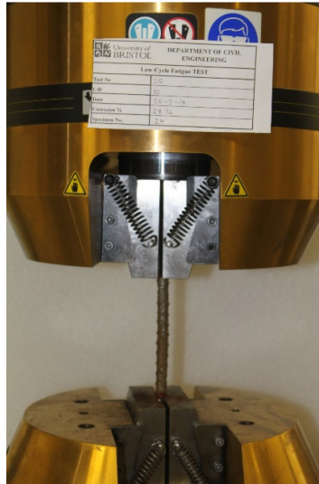
Fig. 4. Low-cycle fatigue test setup of a corroded bar with L/D = 5
