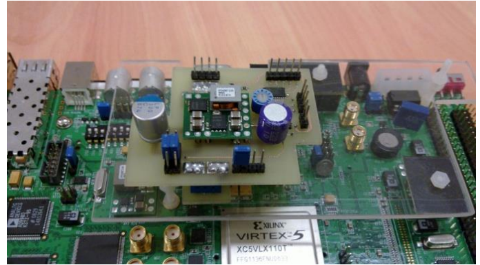
Figure 1. Voltage scaling PCB
