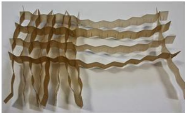
e) The slots on strips are interlocked
