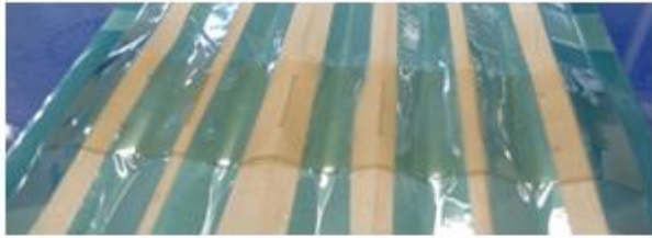
c) Strips are fixed before forming to maximise fold accuracy
