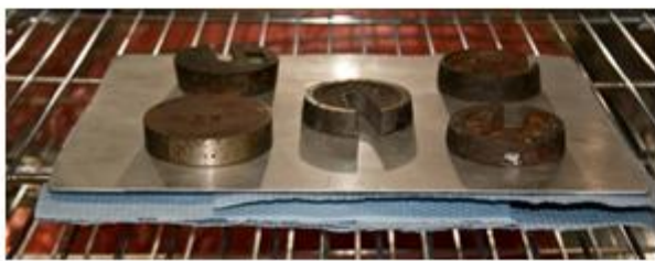
g) Epoxy is cured at 70°C for 1 hour with weights to keep the sample flat
