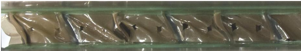
Figure 10: Tearing of the ventilation holes in A-type shear samples
