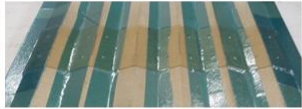
d) Strips after forming in Formech FM1 vacuum forming table
